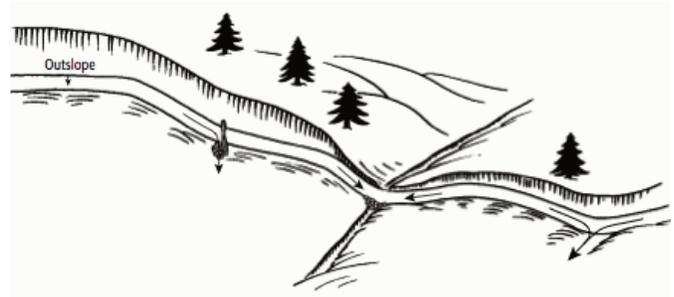
Figure 14-9. A rolling grade uses undulating crests and dips to divert water off the tread.
