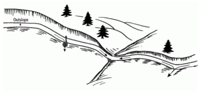
Figure 14-9. A rolling grade uses undulating crests and dips to divert water off the tread.
