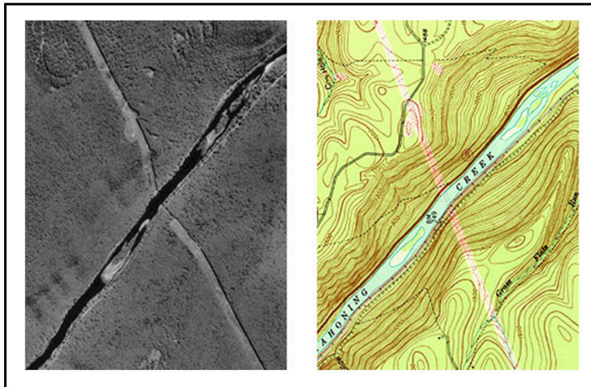
Aerial photogrammetry. Photogrammetry is the process of taking measurements of the ground from photos of the earth in order to make the data necessary for maps. 10
