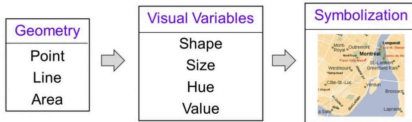
Symbolization components. Basic building blocks of symbolization are geometry (points, lines, and areas) and visual variables (shape, size, hue, and value).<sup>6</sup>
