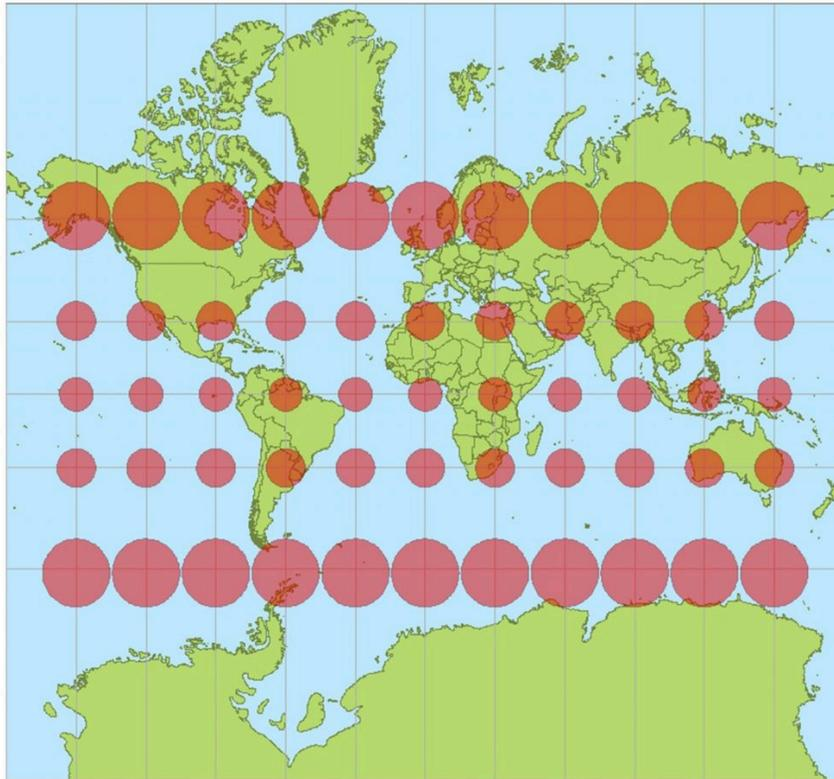
Mercator distortion. The Mercator projection is conformal because it preserves shape and angle but strongly distorts area.<sup>14</sup>
