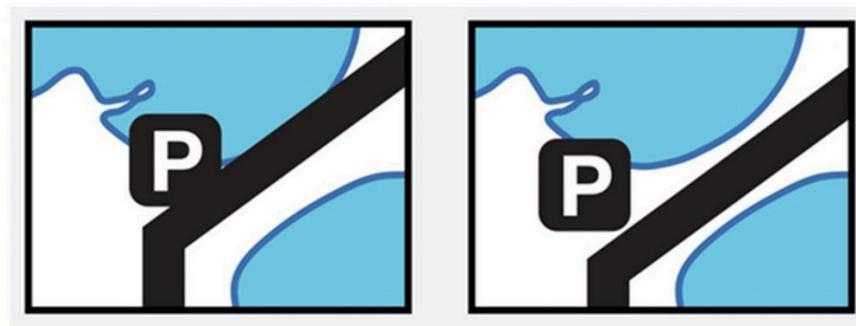
Displace. Map generalized by moving the road to enhance separation from the shoreline. <sup>17</sup>
