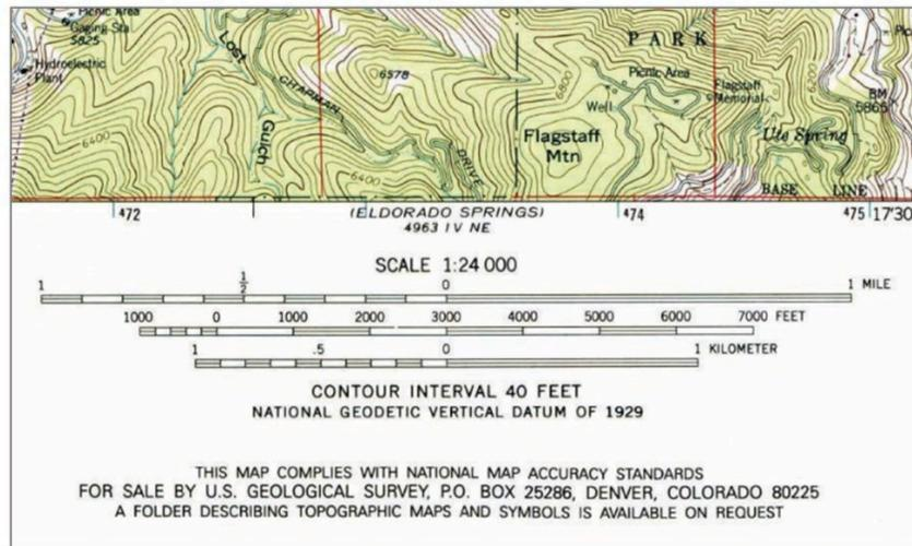
Representative fraction. Representative fraction and scale bars from a United States Geological Survey (USGS) topographic map. This topographic map has an RF of 1:24,000, which means that one unit on the map represents 24,000 units on the ground. <sup>2</sup>
