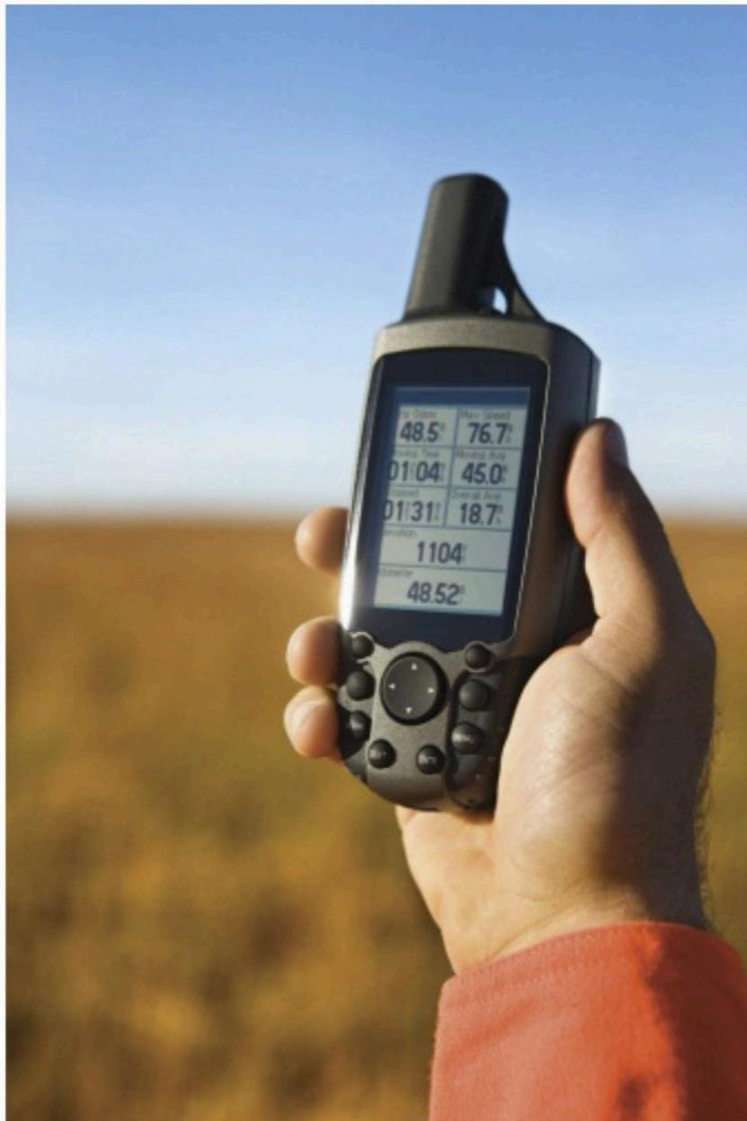
GPS handset. Handsets have specialized radios and computers that receive signals from GPS satellites and then determine location. <sup>5</sup>
