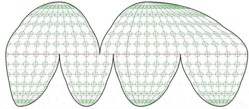
Interrupted distortion. This equal area projection preserves area but distorts shape, but not as much as it would if it were not interrupted.<sup>21</sup>
