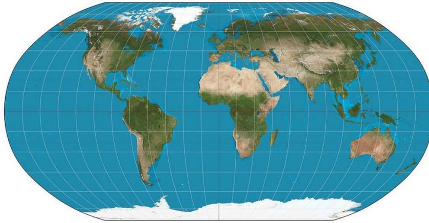
Robinson Projection. Some projections, including the Robinson projection, strike a balance between the different map properties. In other words, they do not preserve shape, area, or distance, but instead try to avoid extreme distortion.<sup>18</sup>
