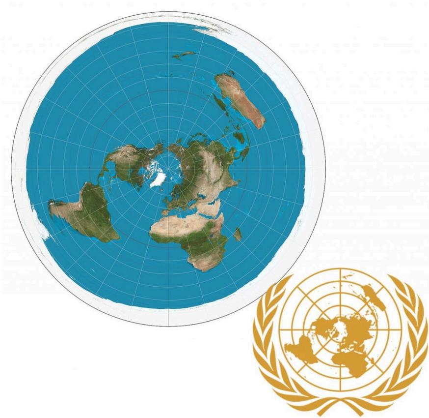
Azimuthal Equidistant projection. In this equidistant projection, all points are the proportionally correct distance and direction from the center point. This projection is used on the map of the United Nations.<sup>17</sup>
