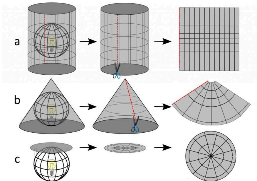
Thinking of projections in physical terms. You can conceptualize projection as working with a clear globe, a light bulb, and tracing paper. If you had a clear globe the size of a beach ball and placed a light inside this globe, it would cast shadows onto a surrounding surface. This surface can be a (a) cylinder, (b) cone, or (c) plane.<sup>10</sup>
