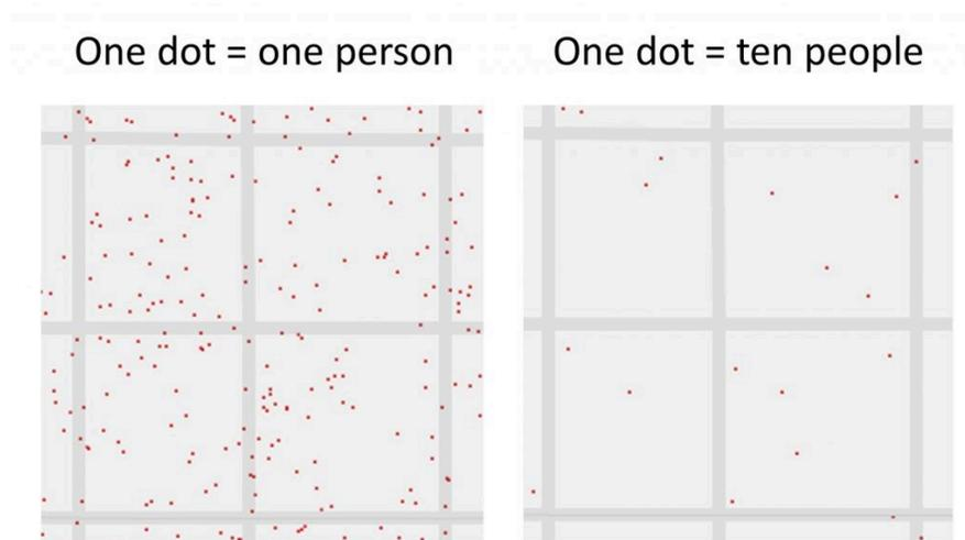
Dot map simplification. The placement of dots in the middle of roads and uneven distribution around the block are evidence that the dots in the one-to-one dot map have been displaced. The many-to-one map of the same blocks simplifies the amount of data shown and places dots at an average location.<sup>5</sup>
