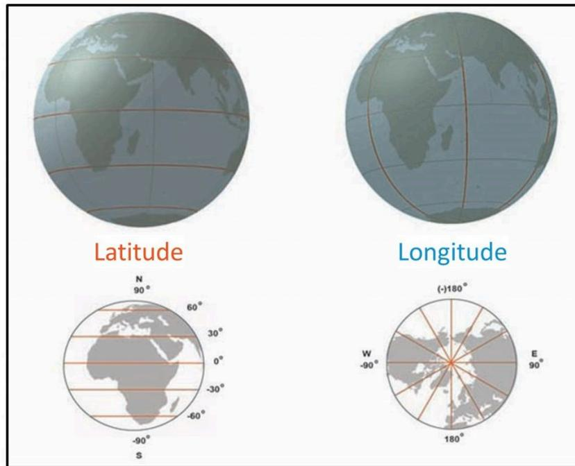
Longitude and latitude. The graticule is based on an east-west scale called longitude and a north-south scale called latitude. <sup>6</sup>
