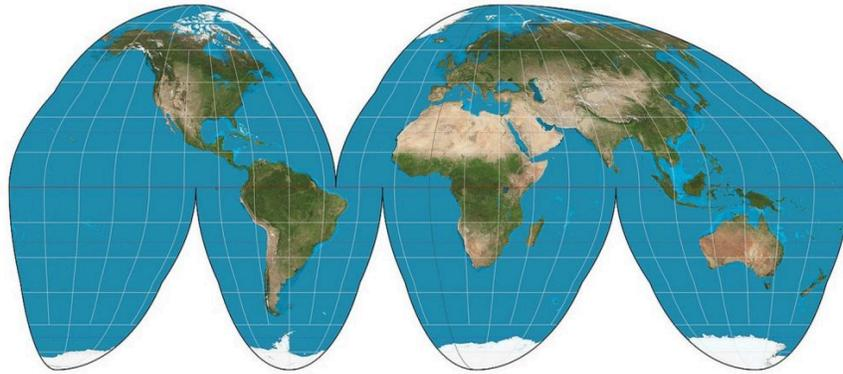
Goode homolosine projection of the world. This equal-area projection is interrupted in the sense that it uses lobes or sections.<sup>20</sup>
