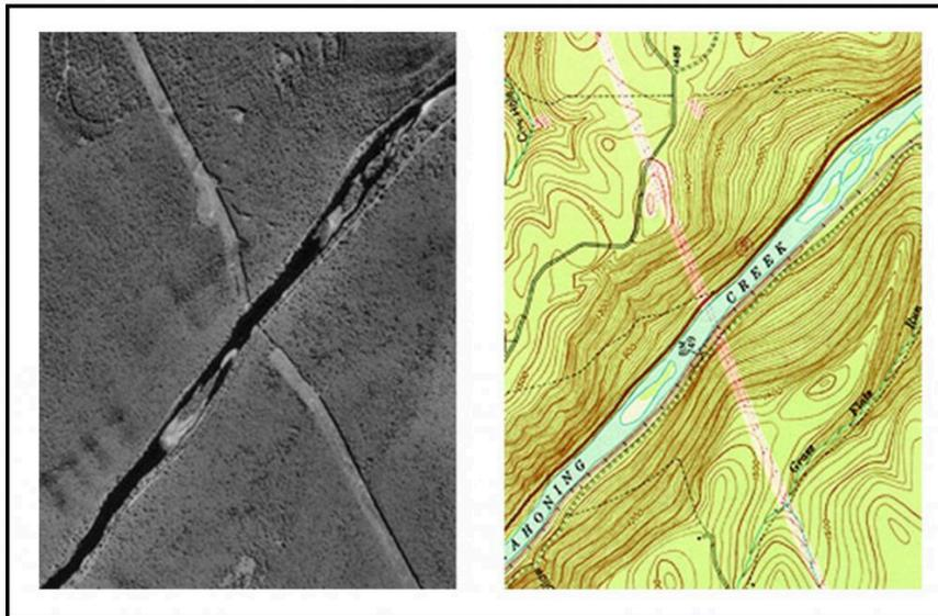
Aerial photogrammetry. Photogrammetry is the process of taking measurements of the ground from photos of the earth in order to make the data necessary for maps.<sup>10</sup>
