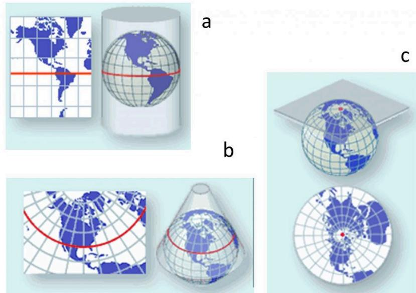
Tangency. Red lines or dots mark the tangent line or point respectively. The flat surface touches the globe and it is the point on the projected map which has the least distortion. The place where the developable surface touches the globe is known as the tangent point or tangent line. These surfaces can be a (a) cylinder, (b) cone, or (c) plane. <sup>11</sup>
