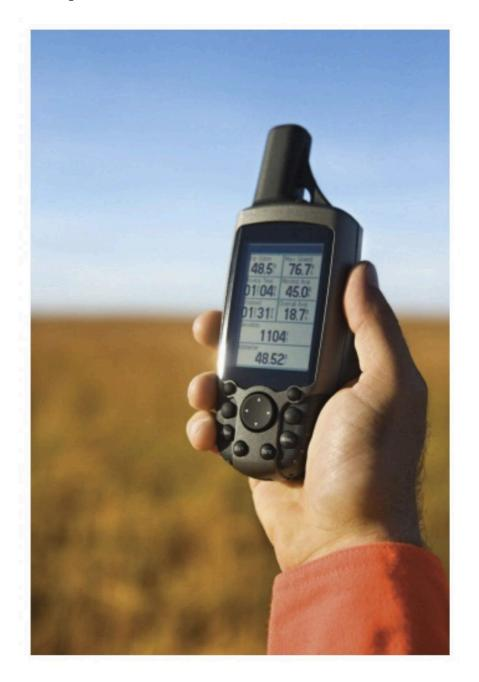
GPS handset. Handsets have specialized radios and computers that receive signals from GPS satellites and then determine location. <sup>5</sup>
